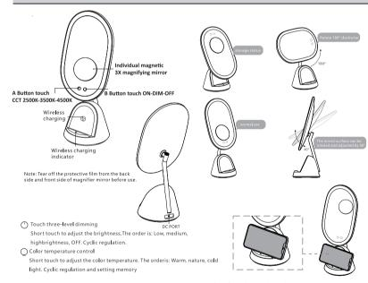
Wireless fast charger board support 10W Max Tips: When the indicator light is red, it is charging, when it is green, it is full, and when the red light is flashing, it is abnormal charging
