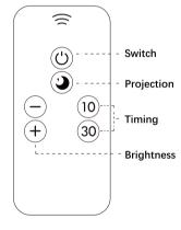
Switch : Press to turn on all lights, then press to switch to breathing light mode, and then press to turn off all lightsOFF position
