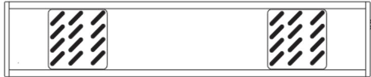
Attach an iron sheet with double-sided tape to the back of the lamp
