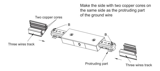
Loosen 2 screw-B on the straight track rail connector, then insert the three-wire tracks into the connector following the arrow direction, and finally tighten all screw-B.
