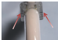
1.6 Ensure that the buckles on both sides of the connector are fully engaged, otherwise poor contact may occur. (as indicated by the red arrows in the above figure, the covers on both sides of the connector should be fully attached to the base without any gaps)
