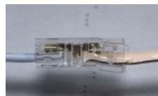
2.3 First, fix the connector cover by hand to avoid misalignment between the MCOB strip and the connector.
