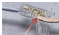
2.2 When inserting the MCOB strip into the connector, ensure that the MCOB strip is fully inserted to avoid poor contact. (indicated by the red arrow in the above figure)
