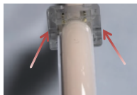
1.6 Ensure that the buckles on both sides of the connector are fully engaged, otherwise poor contact may occur. (as indicated by the red arrows in the above figure, the covers on both sides of the connector should be fully attached to the base without any gaps)
