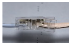
2.3 First, fix the connector cover by hand to avoid misalignment between the MCOB strip and the connector.
