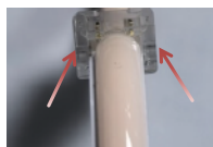
2.5 Ensure that the buckles on both sides of the connector are fully engaged, otherwise poor contact may occur. (as indicated by the red arrows in the above figure, the covers on both sides of the connector should be fully attached to the base without any gaps)
