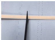
1.1 Cut along the MCOB strip cutting position.
