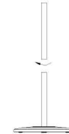
Step 3: Tighten the top tube and middle tube
